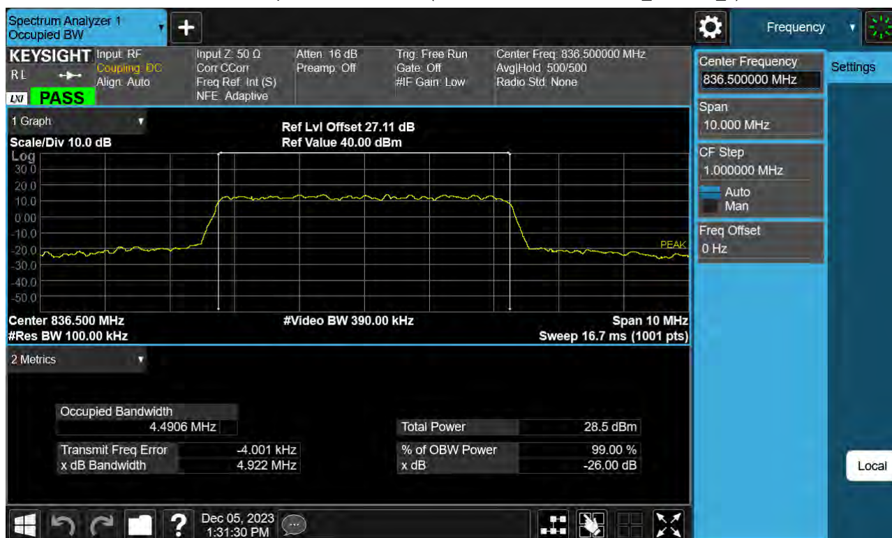
Sub6 n5. Occupied Bandwidth Plot (5 M BW Ch.167300 64QAM_ Full RB _0)
