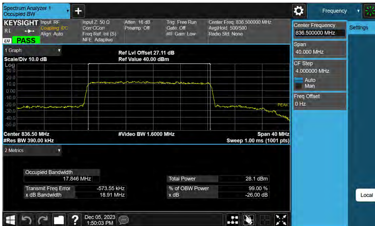
Sub6 n5. Occupied Bandwidth Plot (20 M BW Ch.167300 256QAM_ Full RB _0)
