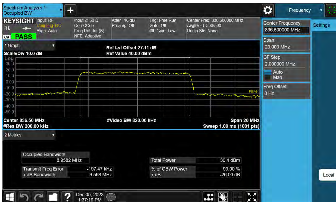
Sub6 n5. Occupied Bandwidth Plot (10 M BW Ch.167300 16QAM_ Full RB _0)
