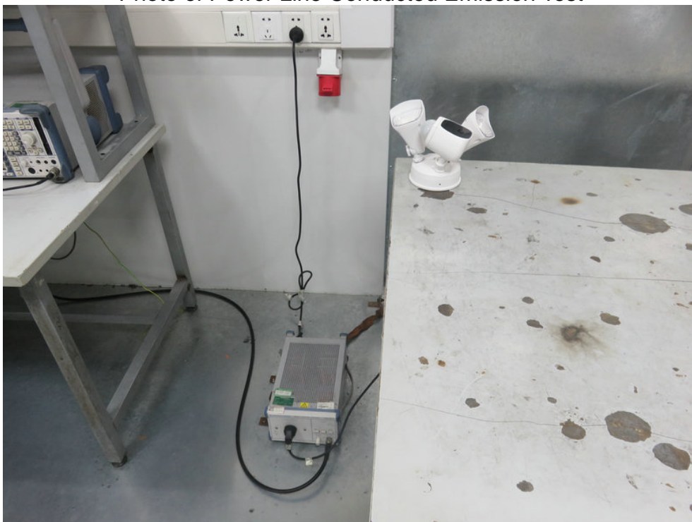
FCC ID: Z63-E97A Photo of Power Line Conducted Emission Test
