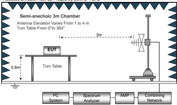
(C) Radiated Emission Test-Up Frequency Above 1GHz
