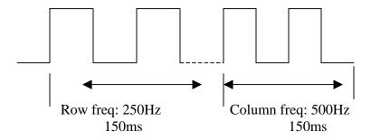
Both waveforms have 50% duty cycle.
