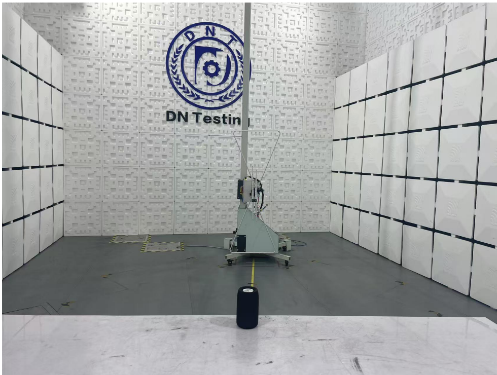
Radiated Emission Test View|(Below 1G)
