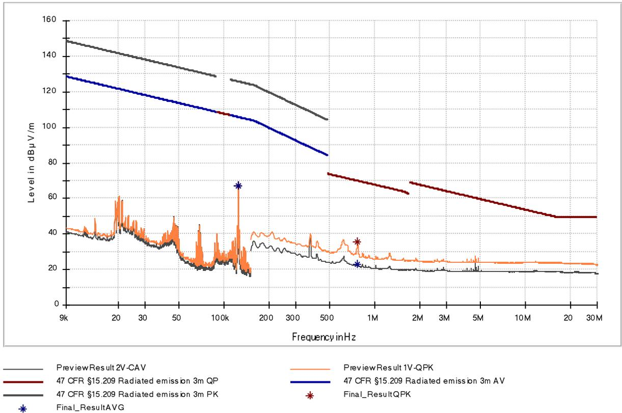
Picture 6: Radiated emission 9 kHz – 30 MHz @ 3m distance
