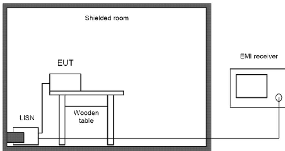
Picture 1: Outline of conducted emission test setup
