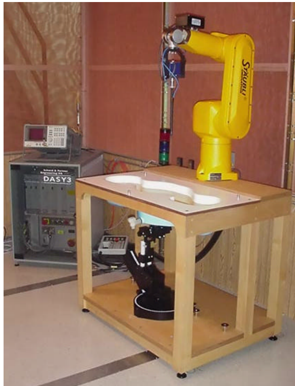
DASY3 SAR Measurement System
