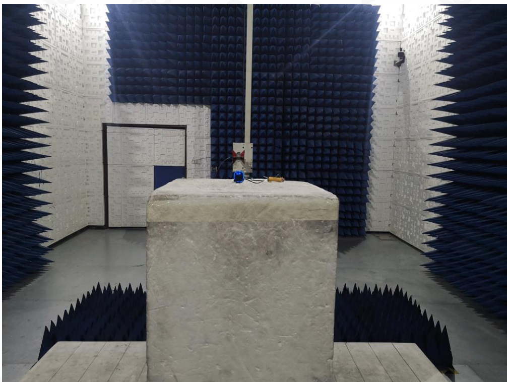
RADIATED EMISSION TEST SETUP ABOVE 1GHZ
