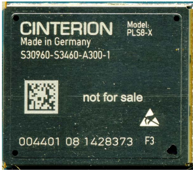
PLS8-X label location lasing on shielding
