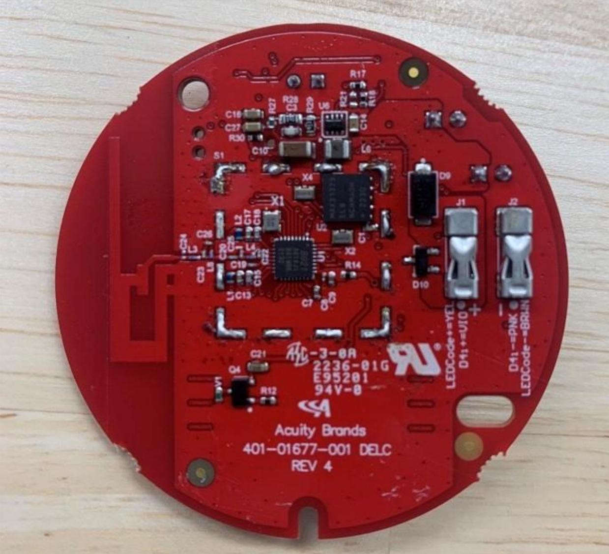
Figure 3: Model LC Top View
