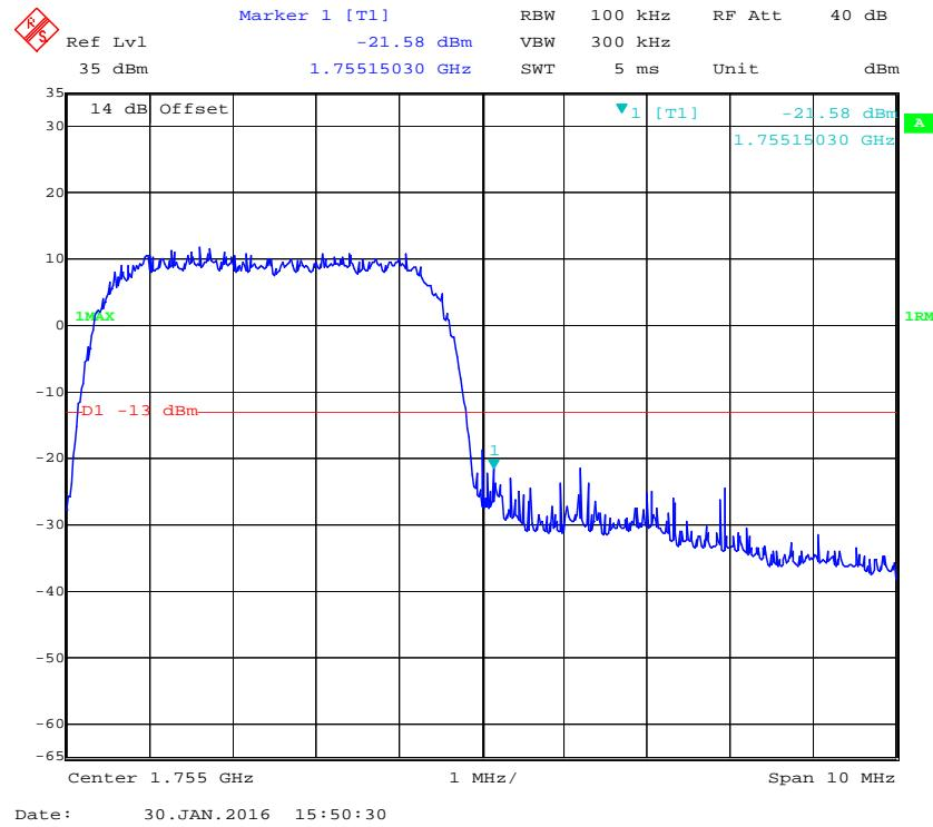
**Band IV, Left Band Edge for HSUPA (BPSK) Mode**
