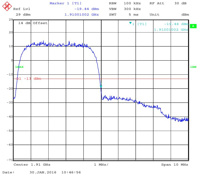
**PCS Band, Left Band Edge for HSDPA (16QAM) Mode**
