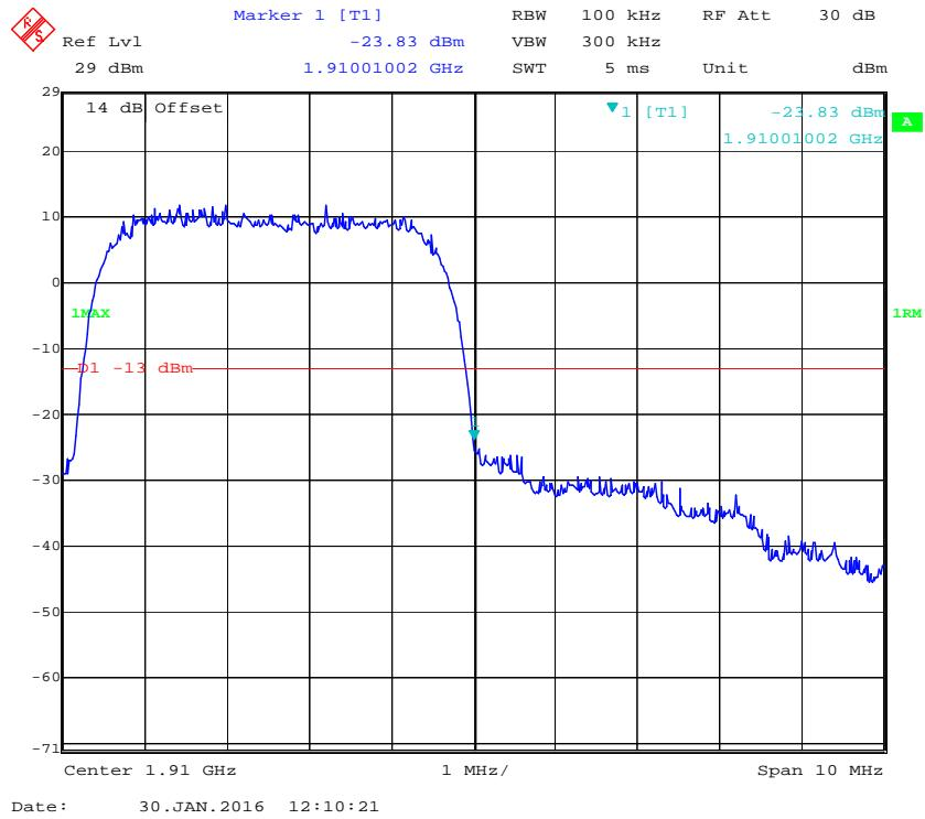
**PCS Band, Left Band Edge for HSUPA (BPSK) Mode**
