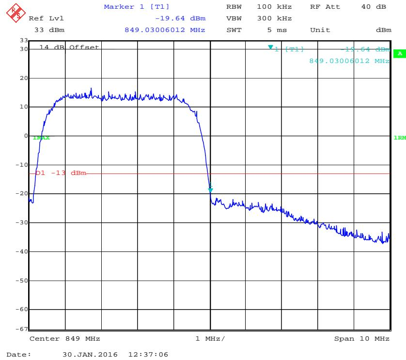
**Left Band Edge for HSDPA (16QAM) Mode**
