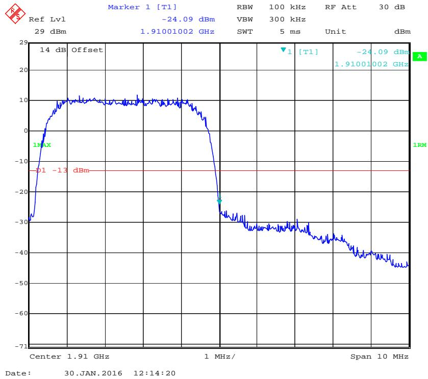
**Band IV, Left Band Edge for WCDMA (BPSK) Mode**
