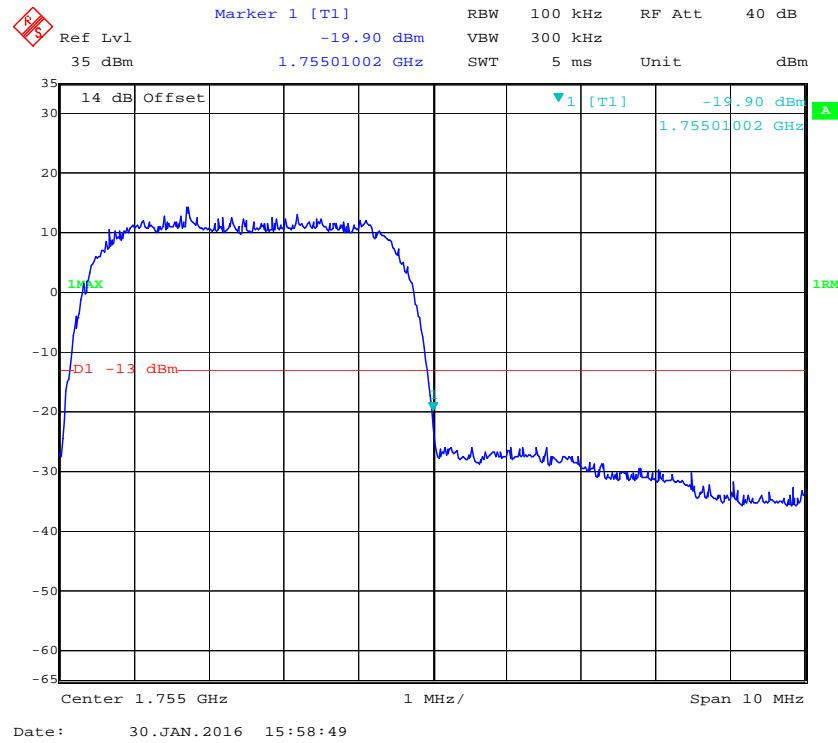
**Band IV, Left Band Edge for HSDPA (16QAM) Mode**
