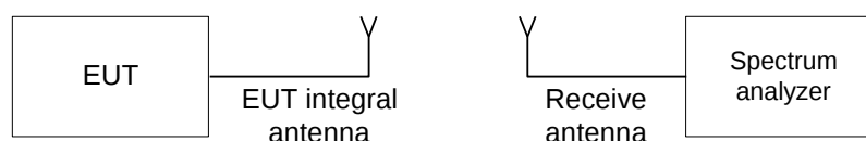
Figure 7.1.1 Setup for transmitter shut down test
