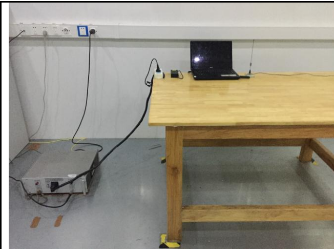
Conducted Emissions Test Setup – Front View
