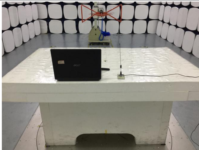
Radiated Emissions Test Setup Below 1GHz
