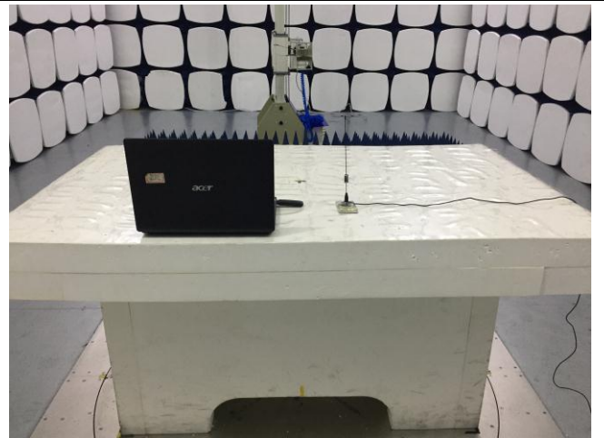
Radiated Emissions Test Setup Above 1GHz
