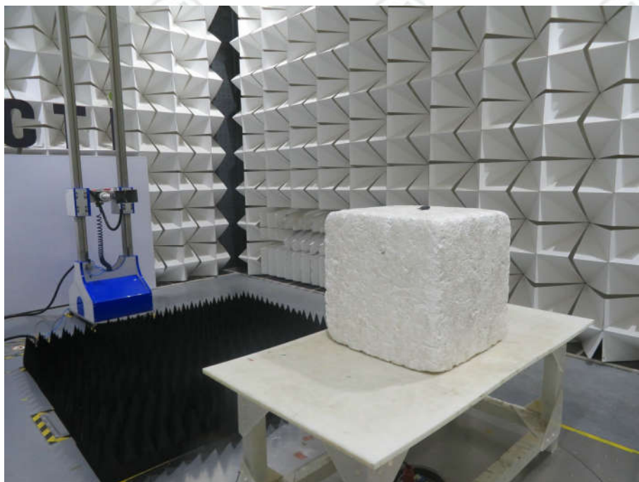
Radiated spurious emission Test Setup-3(Above 1GHz)
