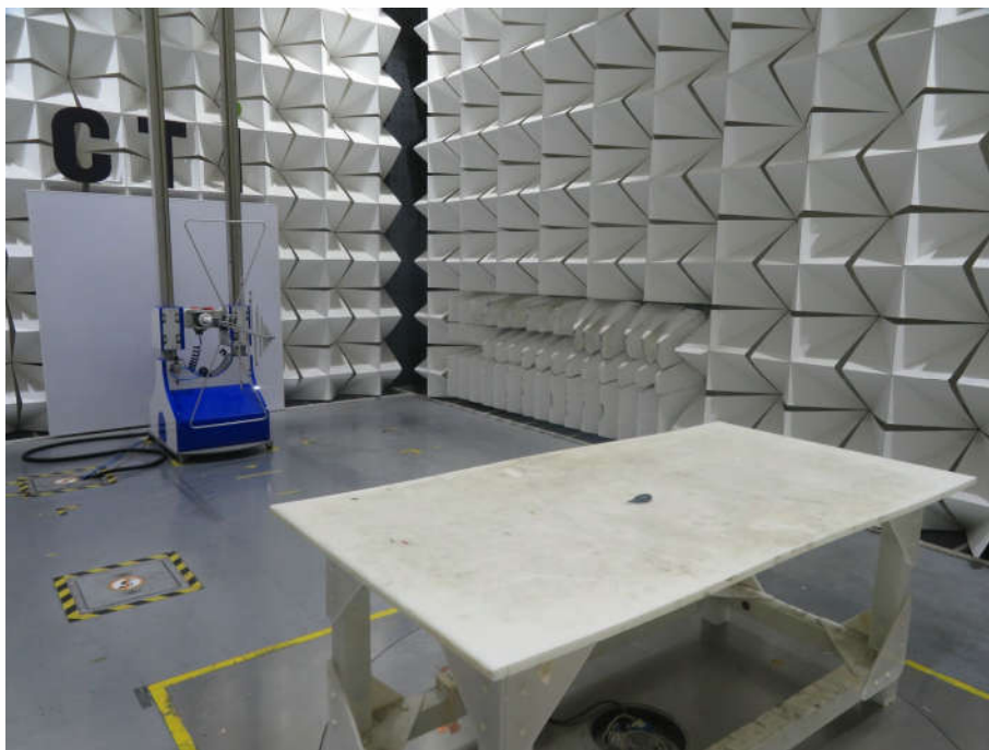
Radiated spurious emission Test Setup-2 (30MHz- 1GHz)
