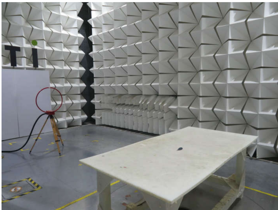
Radiated spurious emission Test Setup-1(Below 30MHz)
