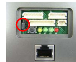
Figure: SWITCH LOCATION
