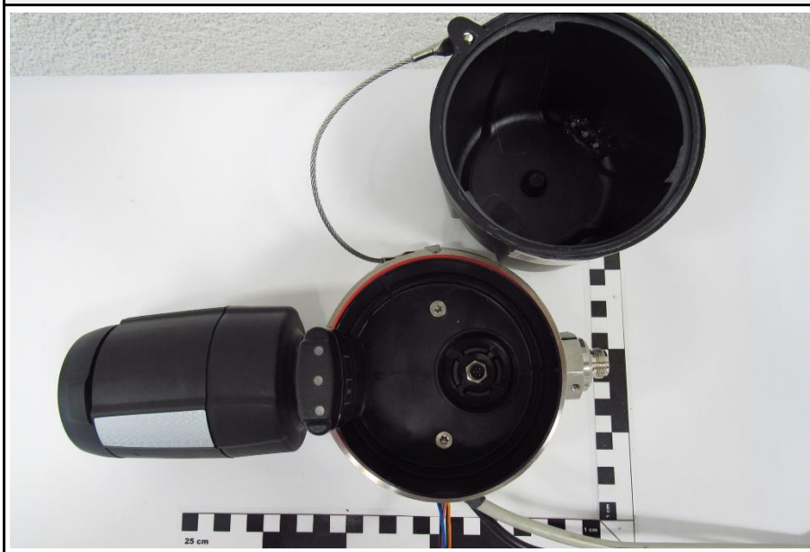
EUT battery housing
