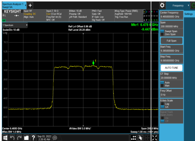
Plot 7-326. Power Spectral Density Plot SDM Antenna 4a (80MHz 802.11ax (UNII Band 6) – Ch. 103, MCS11)
