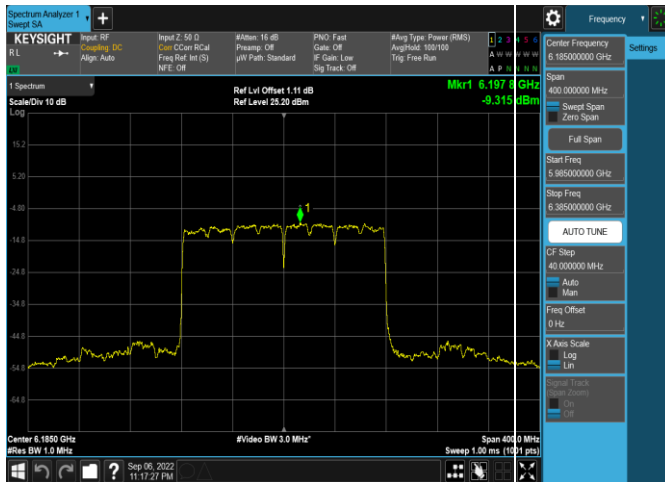
Plot 7-320. Power Spectral Density Plot SDM Antenna 4a (160MHz 802.11ax (UNII Band 5) – Ch. 47, MCS11)
