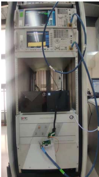
RF Conducted Test setup (BT/WIFI)
