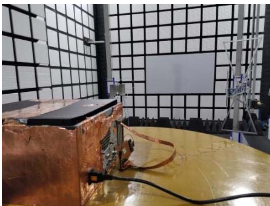
Spurious Radiated Emissions Test setup
