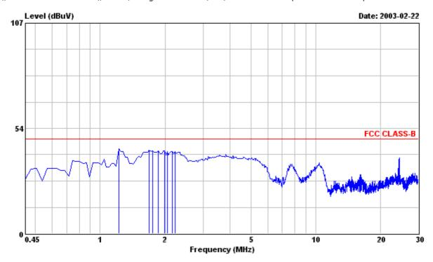
Site : PHILIPS EMI Shielding Room Condition : FCC CLASS-B FCC\_LCI\_L1 LINE
