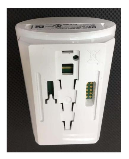
Photograph No.3 PG9914 PIR detector rear side view
