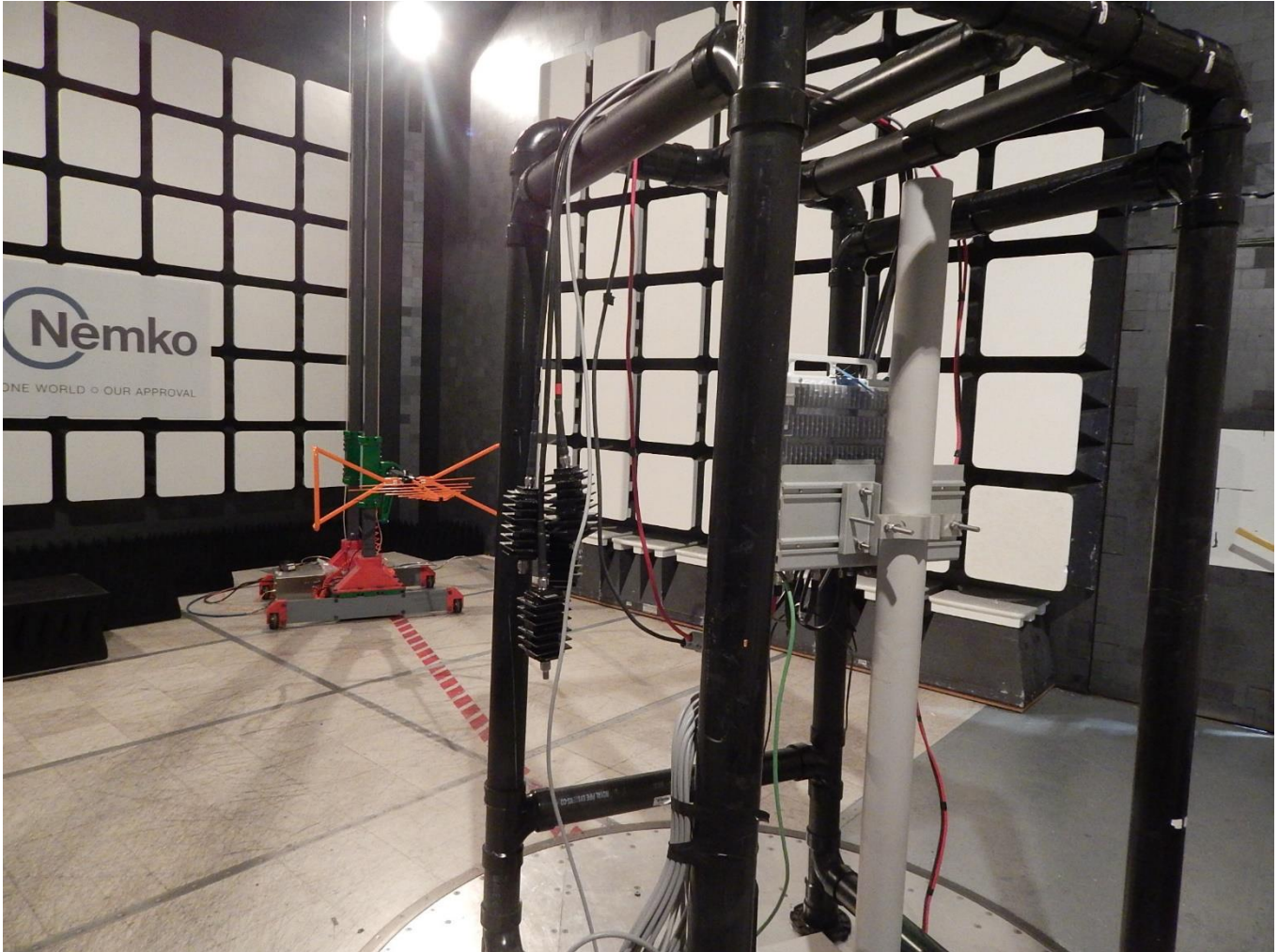
Figure 3.6-4: EUT Set-up for Radiated Compliance Testing
