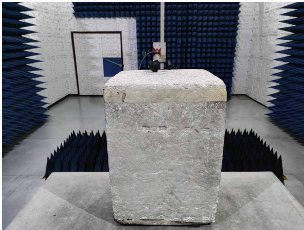
RADIATED EMISSION TEST SETUP ABOVE 1GHz
