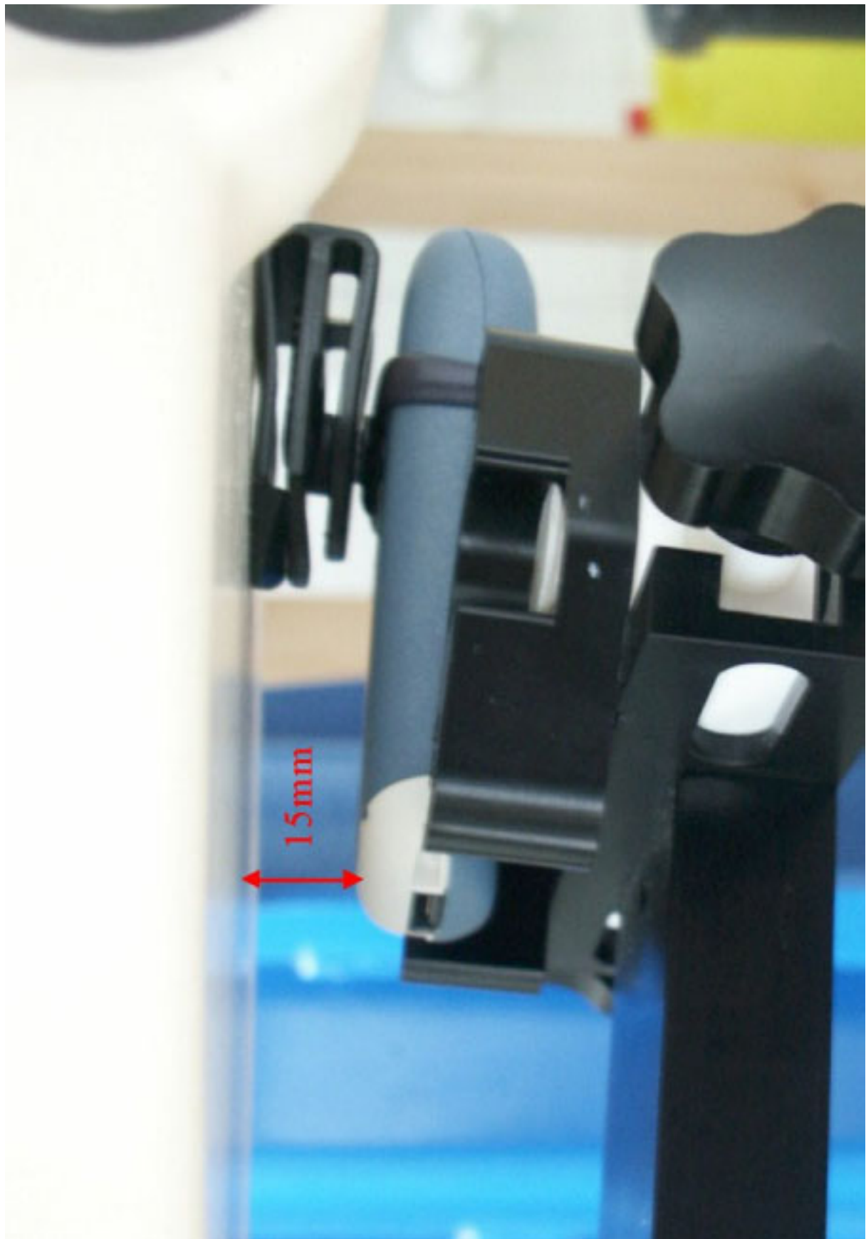
Fig. 28: Body worn configuration, Belt Clip without Headset, GPRS mode (1 TX slot).
