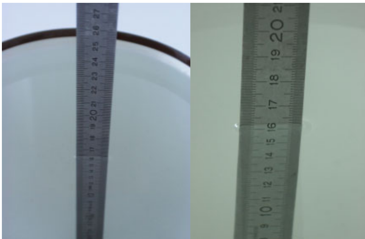
Fig. 30: Liquid depth for PCS 1900 Head and Body measurements.
