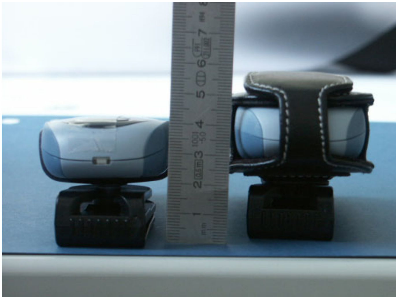
Fig. 21: Phone with tested belt clip and additionally available leather case which dictates a larger distance.
