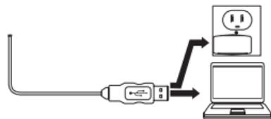
3. Insert the USB charging cable's standard USB plug into the USB port of a computer or suitable 5V 1A USB charging adapter.
