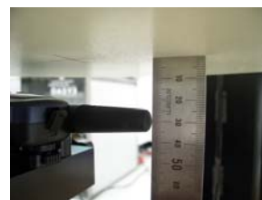
Figure 11. Mouth Face SAR Test Setup
