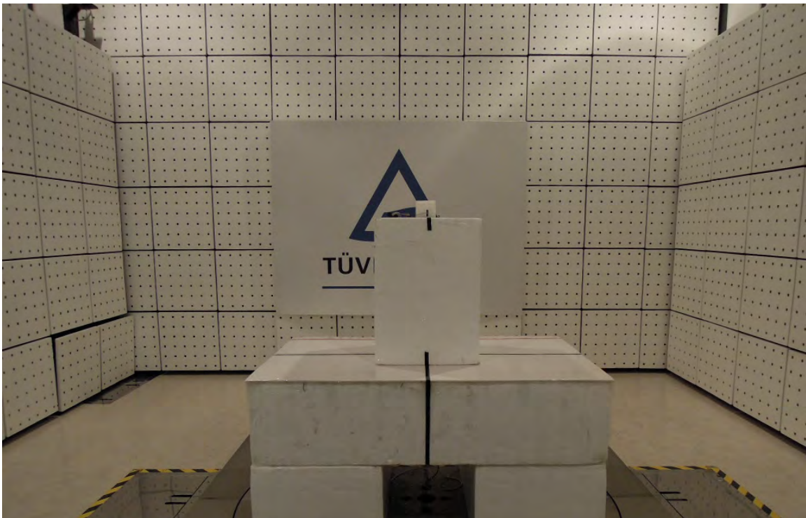
Photograph 23: Set-up for Spurious Emissions (Front View)- 14615300100 -ANT
