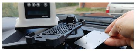
Remove the dash tray or portion of the dash you want to mount to. Screw the multipurpose mount to the top of the dash, then screw the dash plate under the dash to secure the mount in place. This is best suited for a F-150 with removable dash tray to avoid drilling directly into vehicle dashboard.
