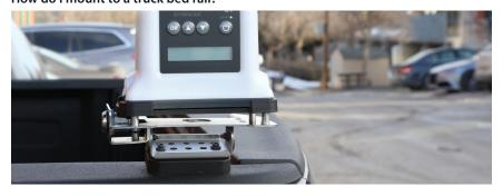
Screw the anchor point into the truck bed rail pop out, and then attach the external bridge mount to the ancho point using screws. Screw the multi-purpose mount to the external bridge mount plate. Slide and snap G7 Bridge into the multi-purpose mount, and lock external bridge mount with key for additional security.
