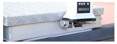
G7 Bridge can be mounted to a truck bed tool box if it has an unobstructed line of sight to the sky. Screw the multi-purpose mount to the external bridge mount plate, and screw the plate to the side of the tool box. Slide and snap G7 Bridge into the multipurpose mount, and lock external bridge mount with key for additional security. Ensure the LCD screen is facing outwards for operation.
