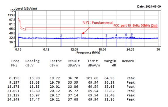
Test Mode: Transmitting(Perpendicular) Tested by: Wlif Wu
