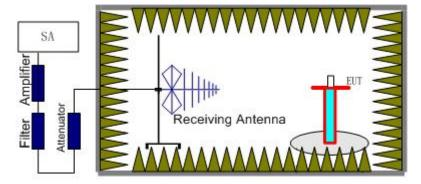
2. The EUT is then put into continuously transmitting mode at its maximum power level during the test. And the maximum value of the receiver should be recorded as (Pr). The placement of EUT is shown in the figure below:
