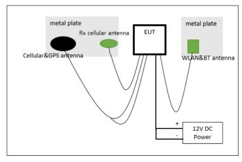
3. The EUT was tested in two states, horizontal and vertical.as show in the attachment.
