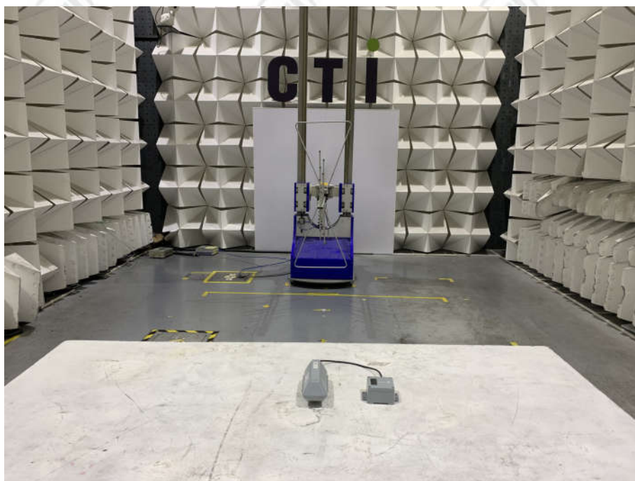
Radiated spurious emission Test Setup-1(Below 1GHz)
