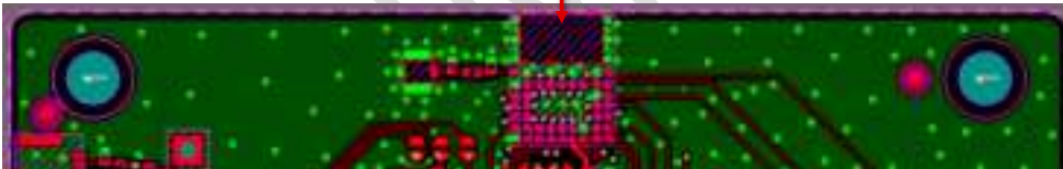
Figure 6: Chip Antenna keep-out area (shown in red) of the BL54L15 \mu development board for the 453-00223 module.
