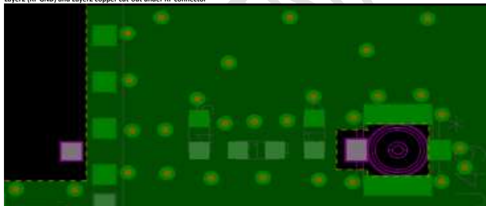
Figure 8: 50-Ohm RF trace design (Layer1 and Layer2) on BL54L15 \mu development board (or host PCB) for use with BL54L15 \mu RF trace pin variant (453-00224) module
