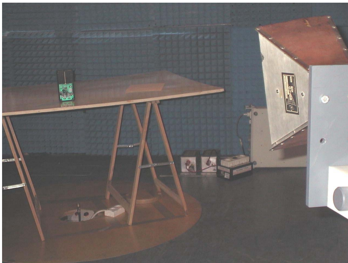
Picture 14.3 Radiated Emission Setup 1GHz-3.5GHz
