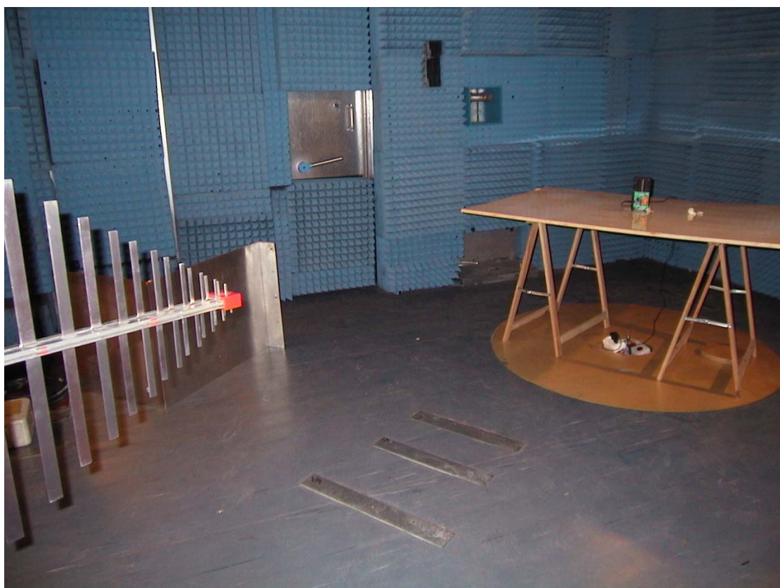
Picture 14.2 Radiated Emission Setup 30MHz-1000MHz
