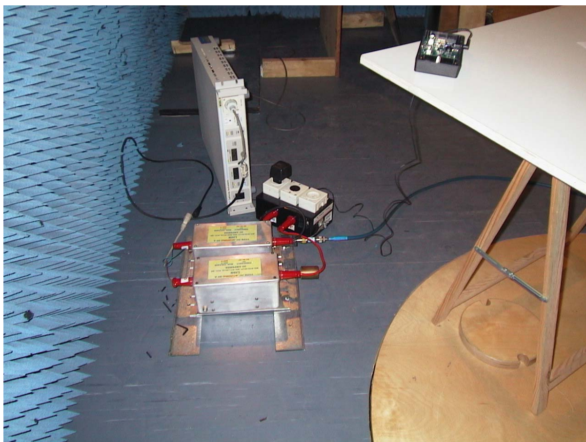
Picture 14.4 Conducted Emission Setup
