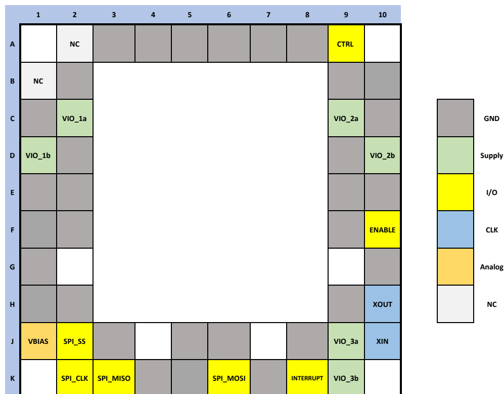
Figure 4.1. Pin configuration of the A111 sensor, top view.
