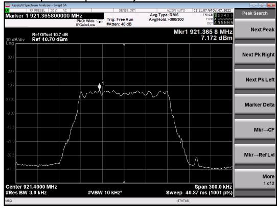
Screen Capture from Spectrum Analyzer: High Channel
