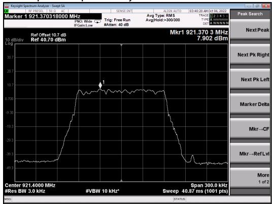
Screen Capture from Spectrum Analyzer: High Channel
