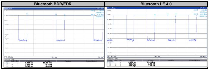
The duty factor of Bluetooth signal has been calculated as following.
