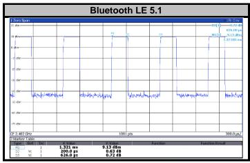
The duty factor of Bluetooth signal has been calculated as following.
