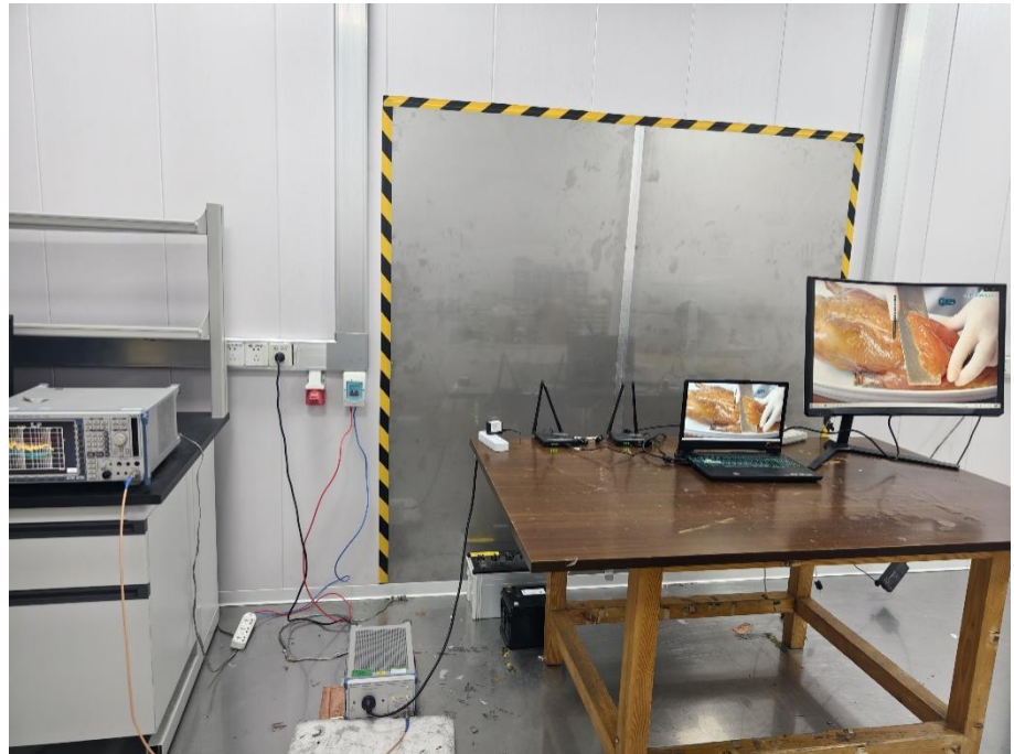
Conducted Emission Test Setup
