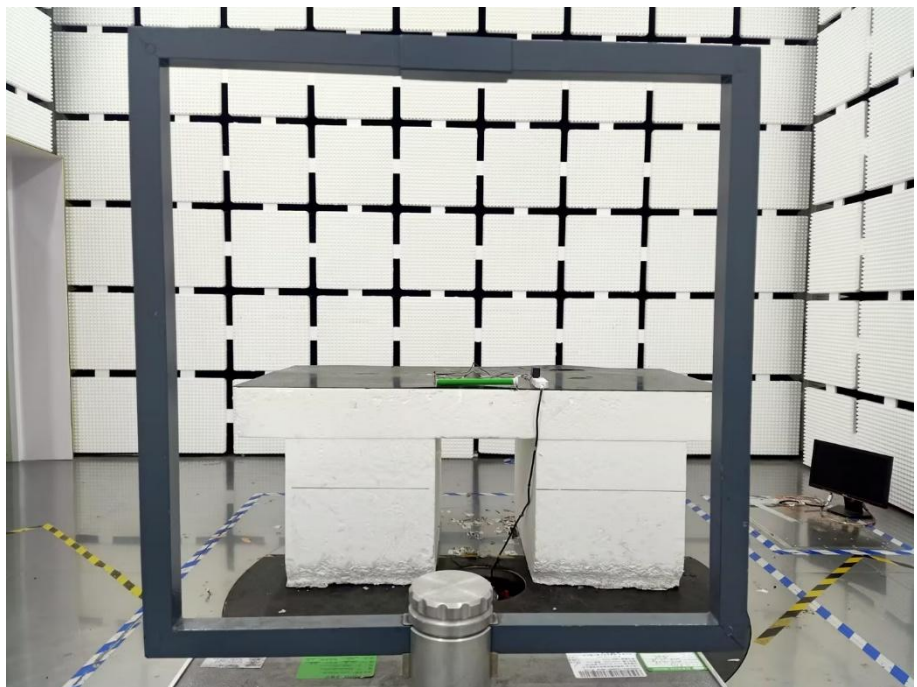
Radiation Emission Test Setup (Below 30MHz)
