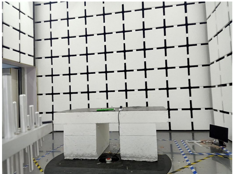
Radiation Emission Test Setup (30MHz to 1GHz)
