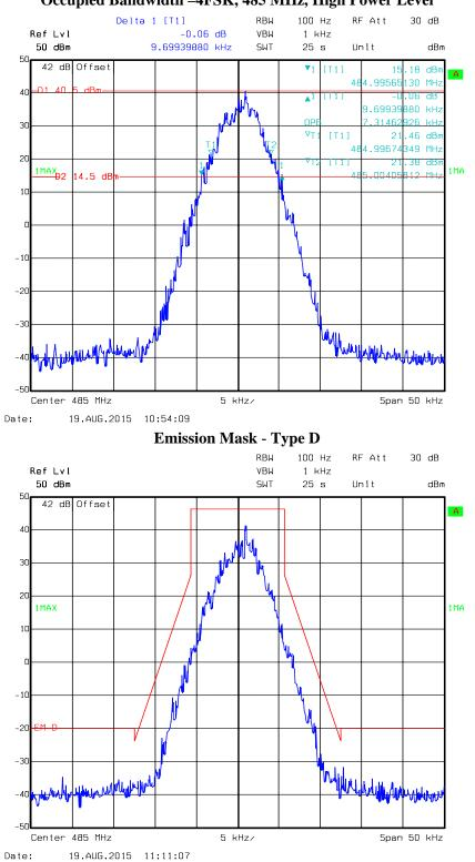
Occupied Bandwidth -4FSK, 485 MHz, High Power Level
