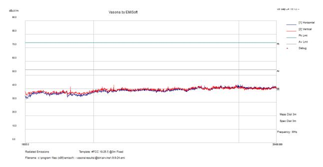
Note: The plot above shows that there were no emissions above the noise floor at 18-26.5GHz frequency range.
