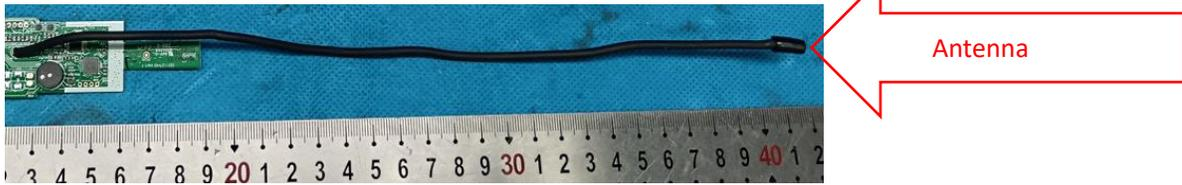
Antenna transmission frequency: 433.92MHz
