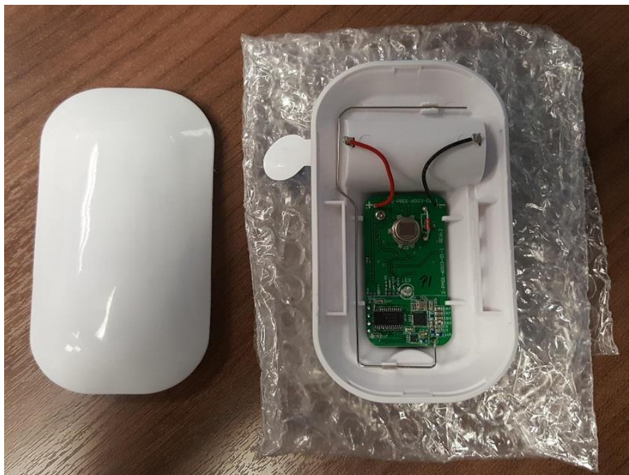
Fig 4: Motion-X Lens Removed, showing PCB Top Side in Plastics with Antenna
