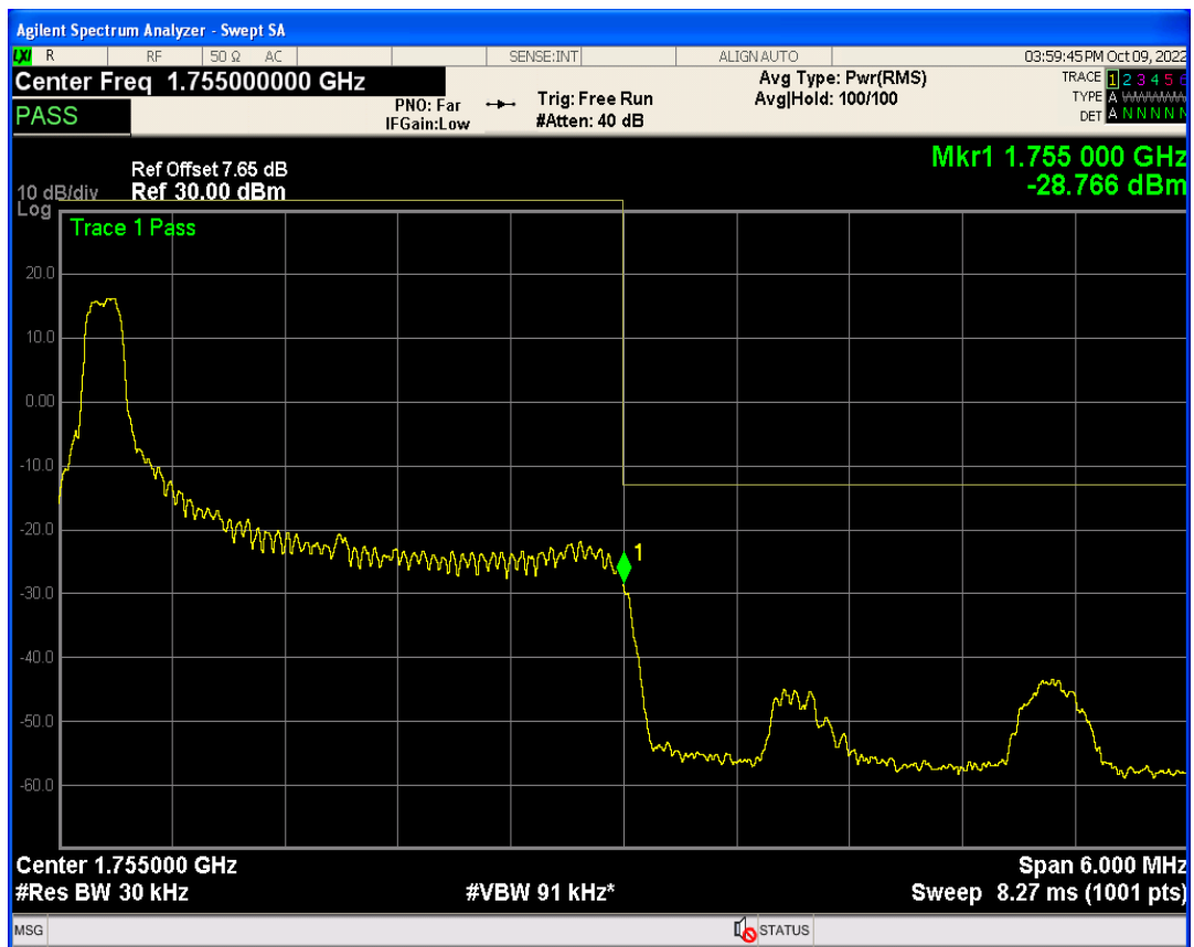
Band4 QPSK BW=3MHz Channel=20385 RB Size=1 Position=#Max
