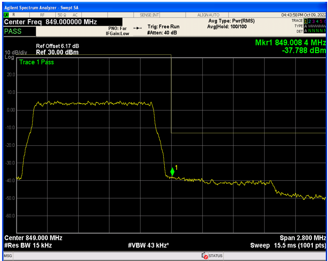
Band5 QAM16 BW=1.4MHz Channel=20643 RB Size=1 Position=#Max
