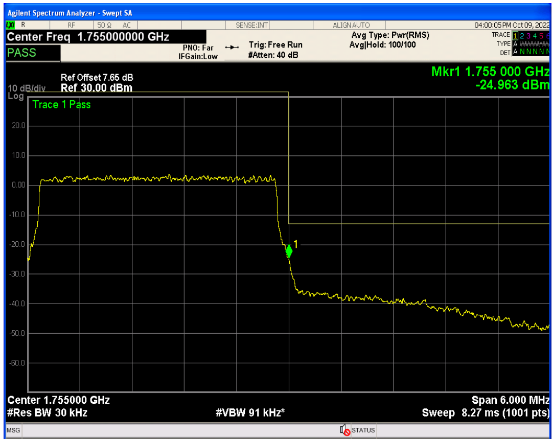
Band4 QPSK BW=5MHz Channel=19975 RB Size=1 Position=#0
