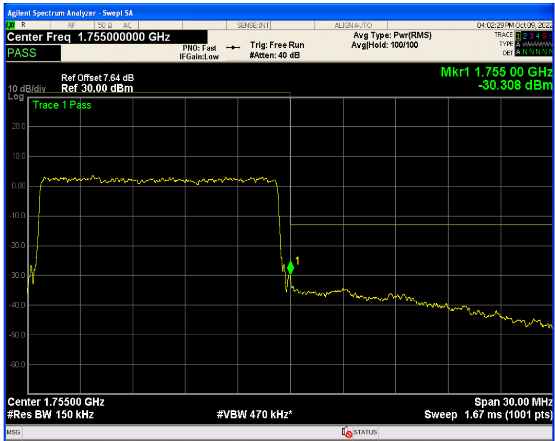
Band4 QPSK BW=20MHz Channel=20050 RB Size=1 Position=#Max
