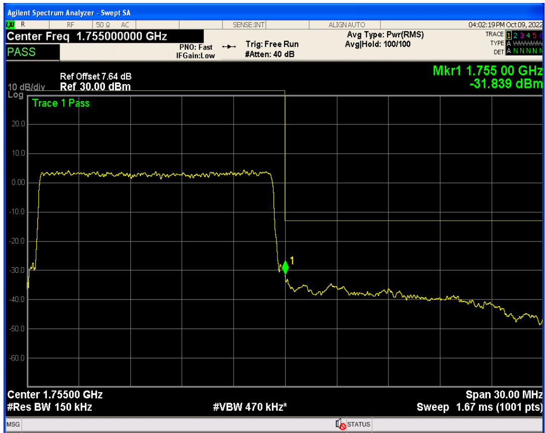
Band4 QPSK BW=15MHz Channel=20325 RB Size=1 Position=#Max
