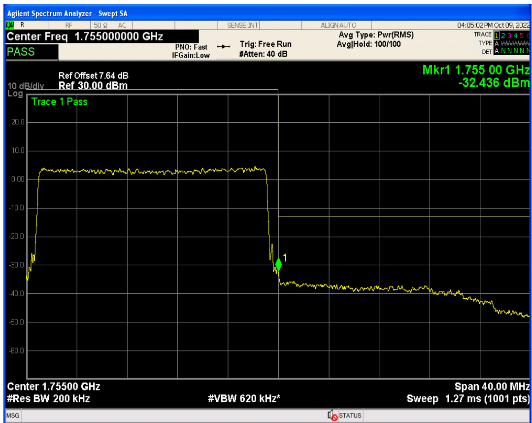
Band4 QAM16 BW=20MHz Channel=20300 RB Size=1 Position=#Max
