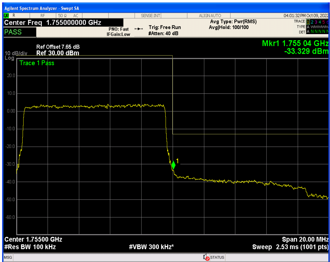
Band4 QAM16 BW=10MHz Channel=20350 RB Size=1 Position=#0
