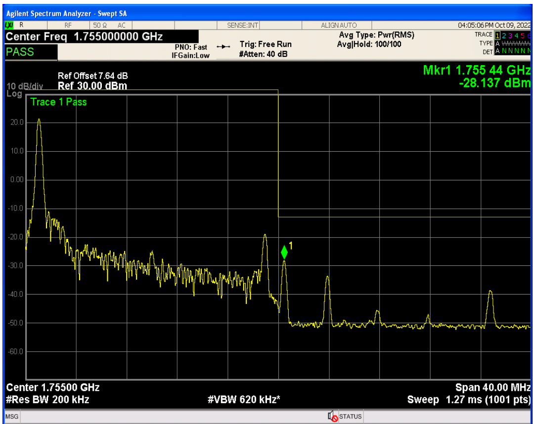
Band4 QAM16 BW=20MHz Channel=20300 RB Size=100 Position=#0
