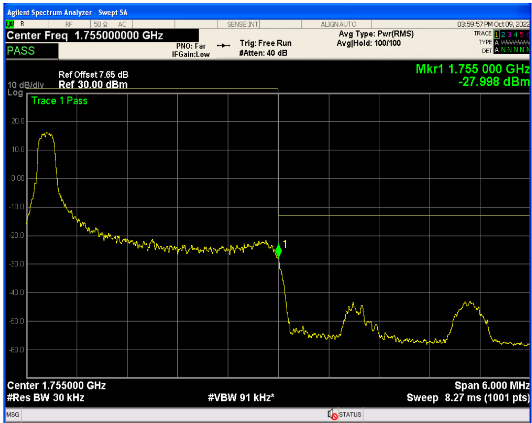
Band4 QAM16 BW=3MHz Channel=20385 RB Size=1 Position=#Max
