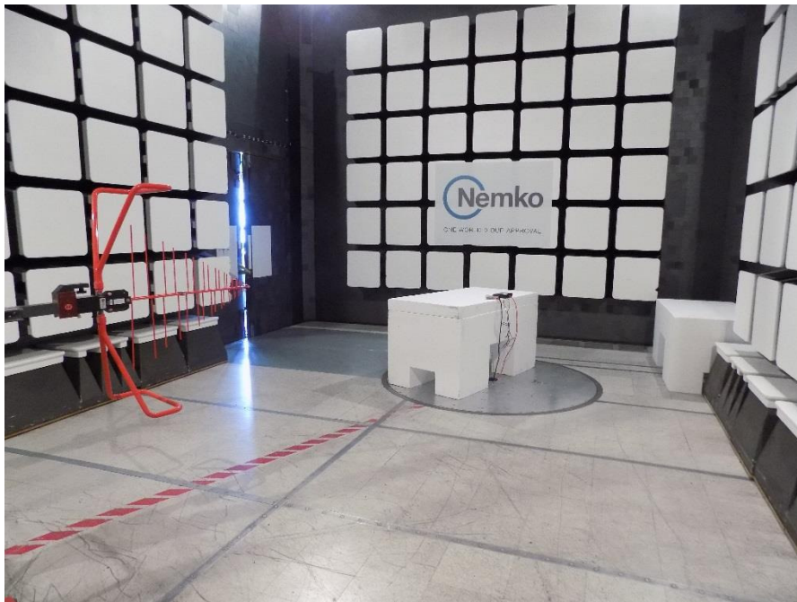
Figure 8.1-1: Radiated spurious emissions setup photo – 30 to 1000 MHz
