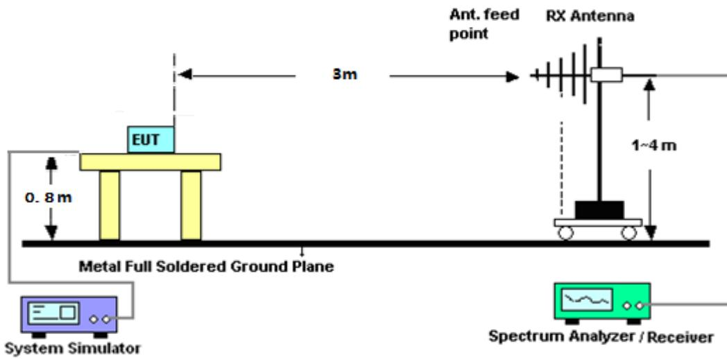
For radiated test from above 1GHz
