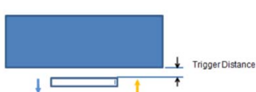
Picture: Proximity sensor triggering distances assessment (Front/Back side)
