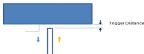
Picture: Proximity sensor triggering distances assessment (Top edge)
