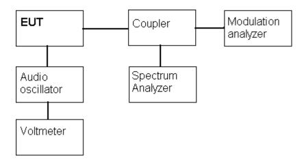
The antenna of the EUT is coupled to the spectrum analyzer and to the modulation analyzer with a near field probe.
