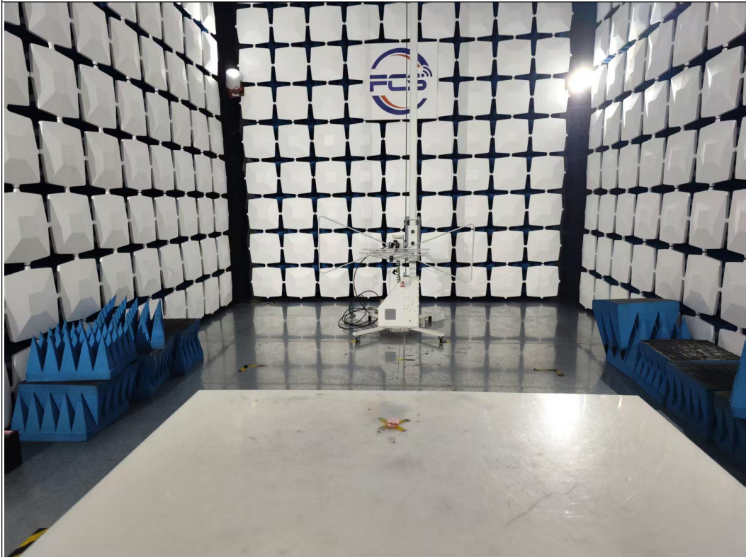
Above 1GHz for radiated emission test setup
