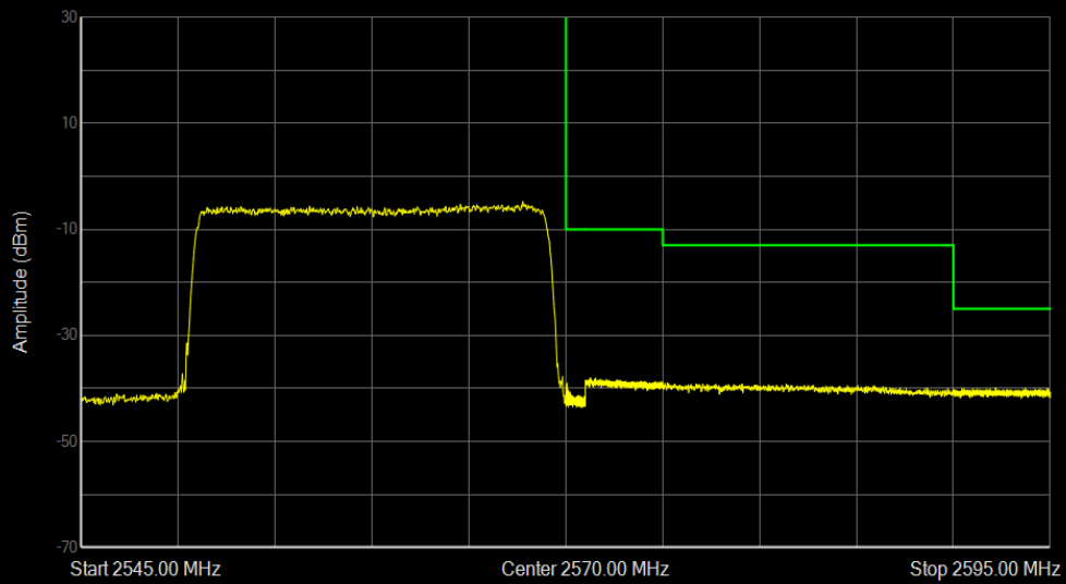
Band7 QPSK BW=20MHz Channel=21350 RB Size=100 Position=#0
