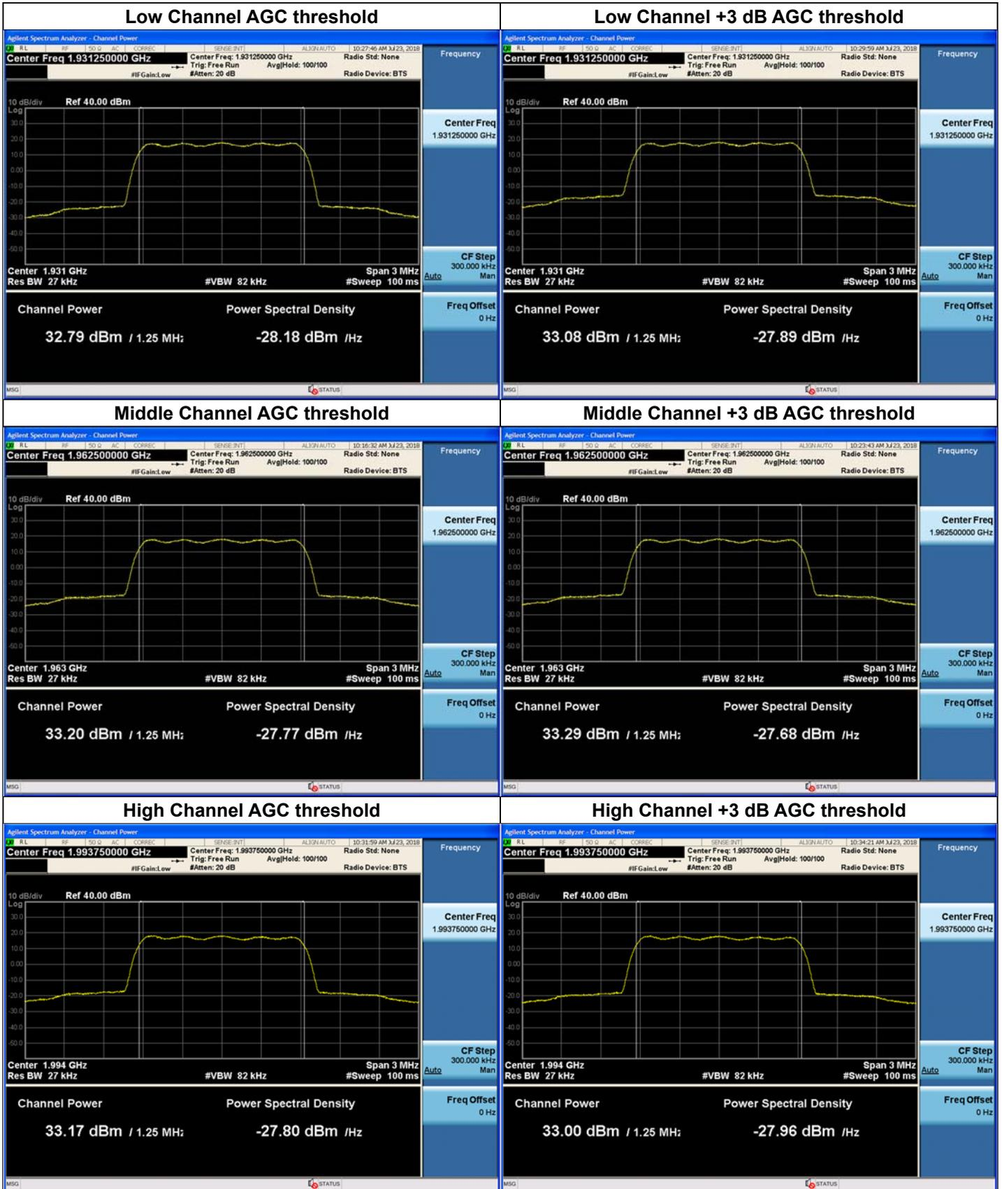
**Plots of RF Output Power for 1900 PCS Band GSM**
