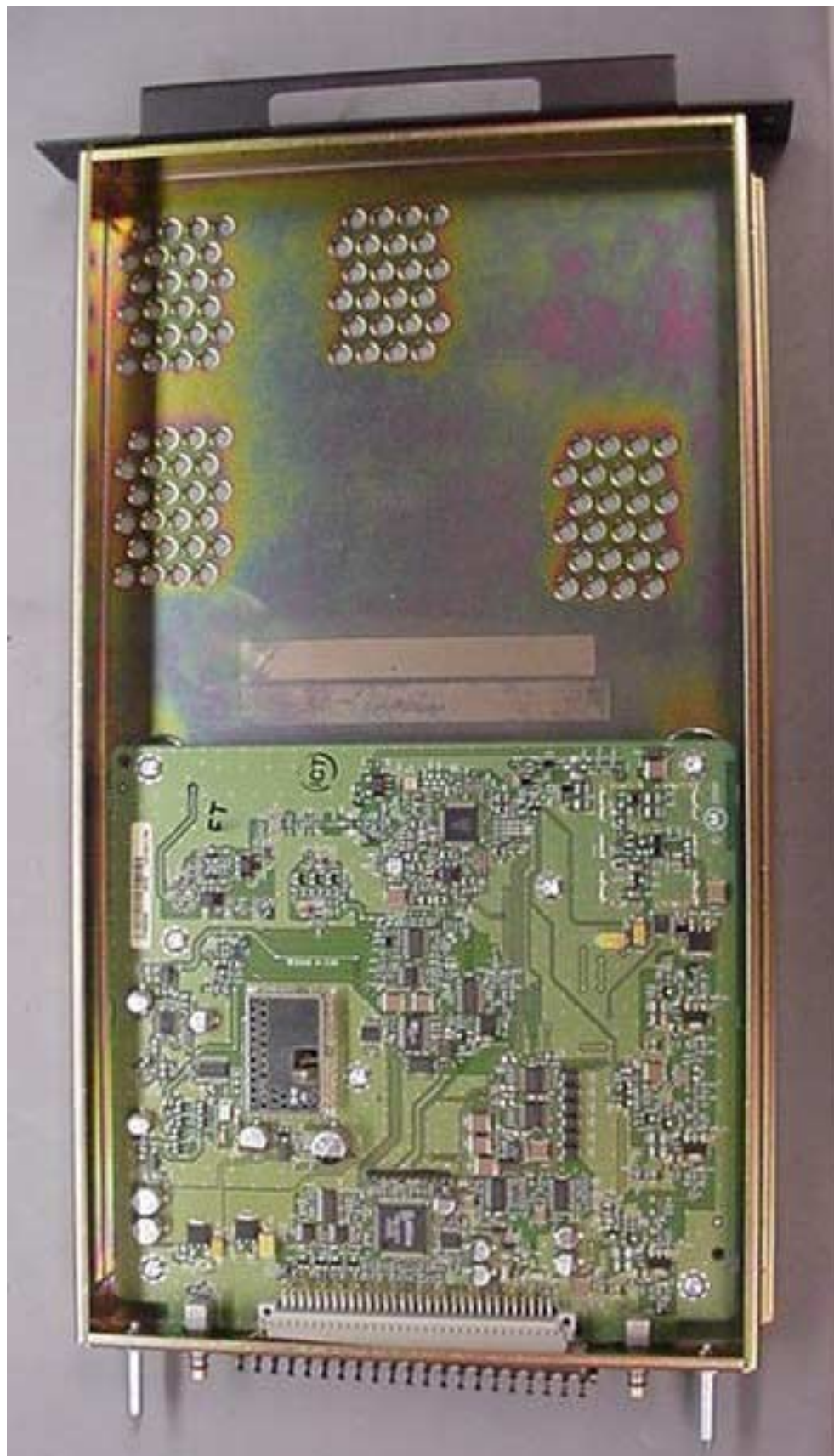
Exciter Module, Component Side
