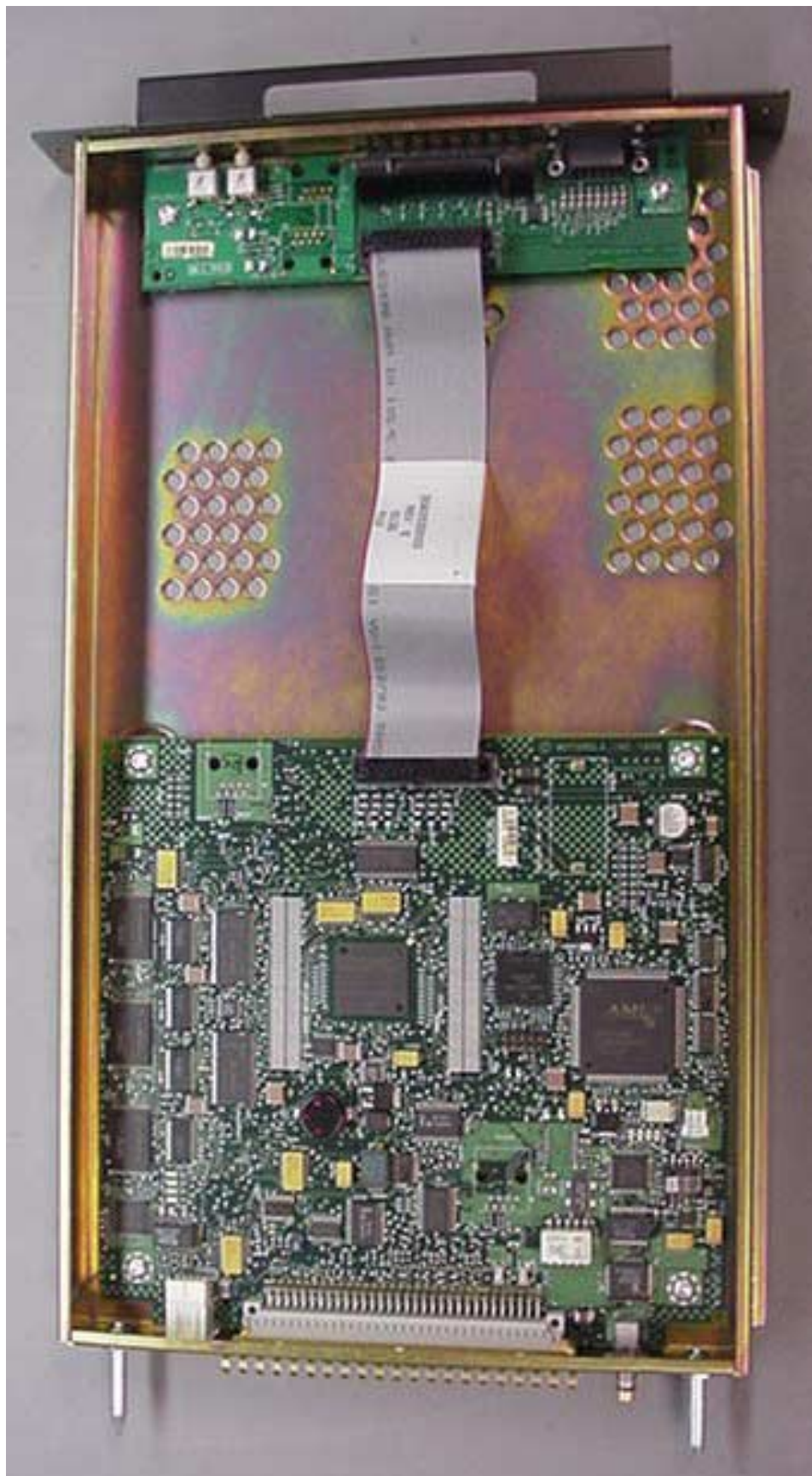
Base Radio Control Module, Component Side
