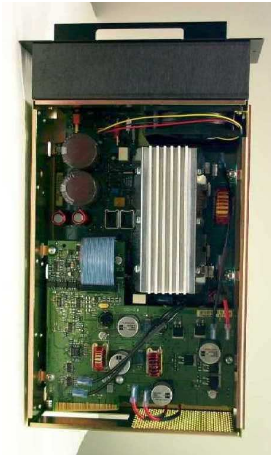
Power Supply Module, Cover Removed
