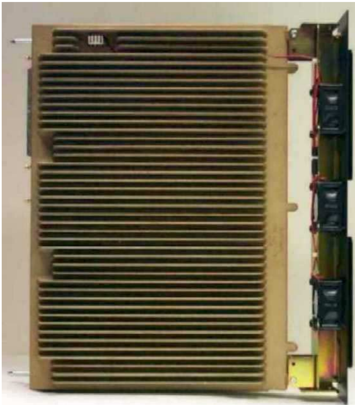
Power Amplifier Module, Heat Sink View
