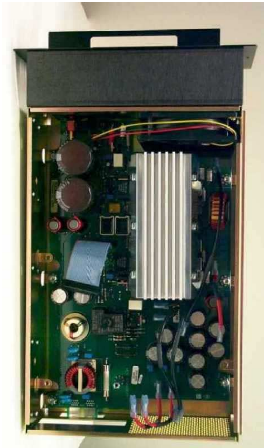
Power Supply Module, Component Side, Sub Board Removed
